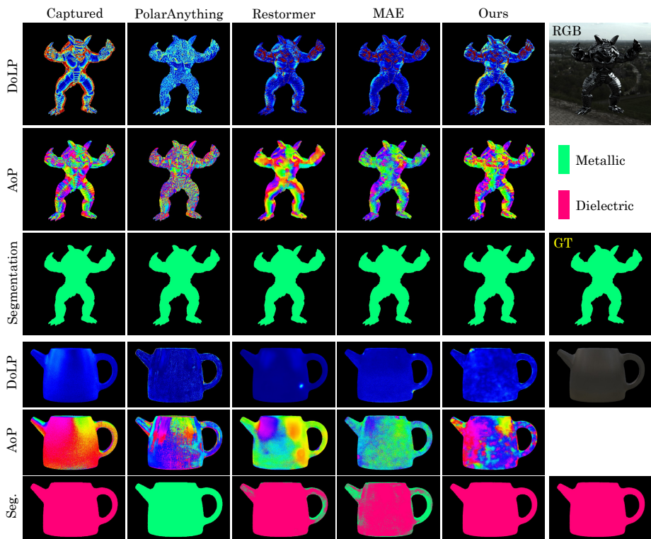
Fig. S9: Additional qualitative results for material detection. Although the predicted AoP is not always visually perfect, the final material masks remain highly accurate, indicating that this task is more strongly driven by polarization magnitude cues.
