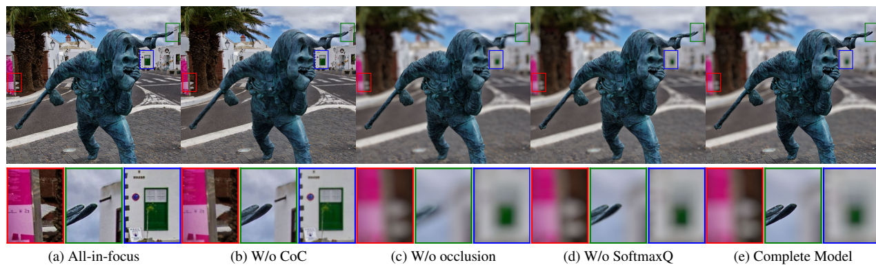
Figure S9. Visual comparisons of the ablation study. The setting of “SoftmaxQ”, “CoC”, and “occlusion” are short for the energy-conserved normalization, circle of confusion constraint, and self-occlusion respectively.
