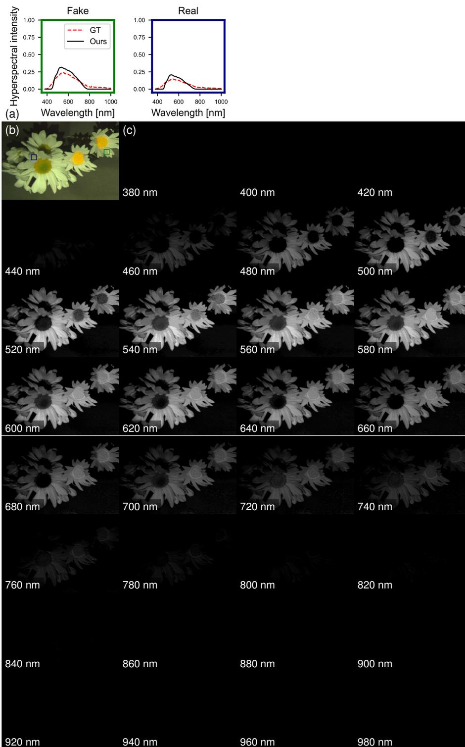
Figure 16. Evaluation of metamer samples of real (left) and fake (right) white daisies. (a) Spectra of metamer samples against ground truth measurements, highlighting the system's ability to capture subtle spectral differences. (b) The reconstructed hyperspectral image in sRGB. (c) Estimated hyperspectral images.
