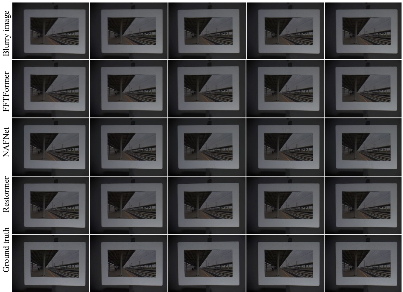
Figure S3-74: Deblurring results for different motion speed. The horizontal value indicates the rotation period of the picture plate. The lower the value, the more serious the motion blur.
