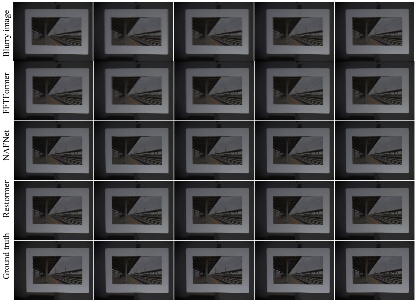
Figure S3-73: Deblurring results for different motion speed. The horizontal value indicates the rotation period of the picture plate. The lower the value, the more serious the motion blur.
