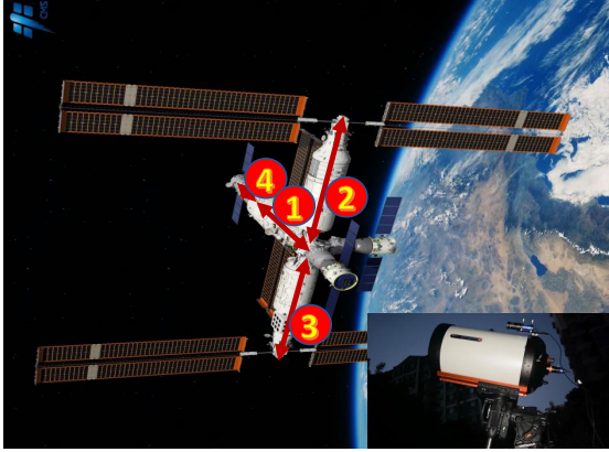
Fig. 11: The Chinese Space Station (CSS) and the imaging instrument. On the left, the official schematic of the CSS, featuring four primary modules: 1 - Tianhe Core Module, 2 - Mengtian Laboratory Module, 3 - Wentian Laboratory Module, and 4 - Tianzhou-6 Cargo Spacecraft. In the lower right corner, the Celestron C14HD telescope paired with a QHY5III678M planetary camera.
